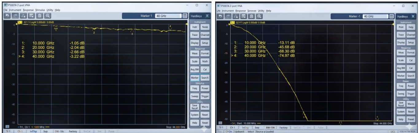
Figure 1: Cavity resonance suppression of absorber (wideband)
