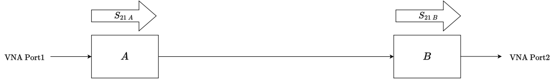
Figure 4: Simplified Flow Diagram of Zero-Length Thru calibration measurement
